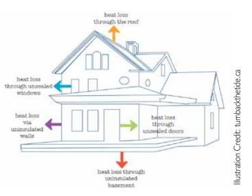
Insulation in walls, exposed ceilings, and attics must be addressed in order to improve the R-value (measurement of thermal resistance) of your home.
